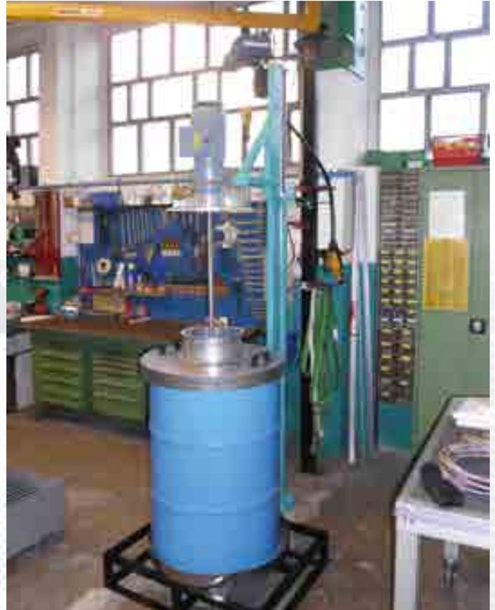
Agitator station, optionally for IBC and 200 liters drum, here 200 liters drum adapter
