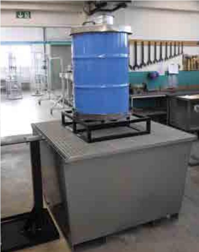
Support structure container agitator station with 1000 liters pan
