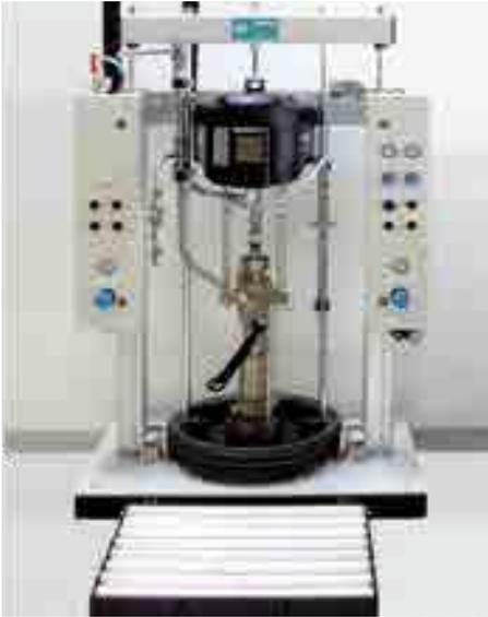
Drum pump station with roller table **Part No. K 68 207 112 31**
