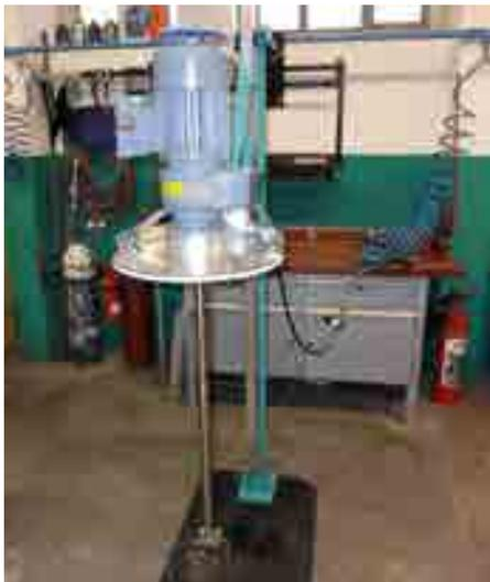
IBC container agitator with sealed cover and folding agitator element
