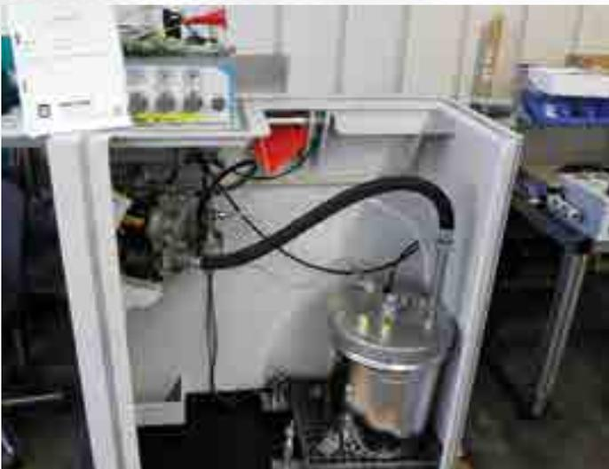
Insulating cabinet with rocker for level monitoring in high-voltage range
