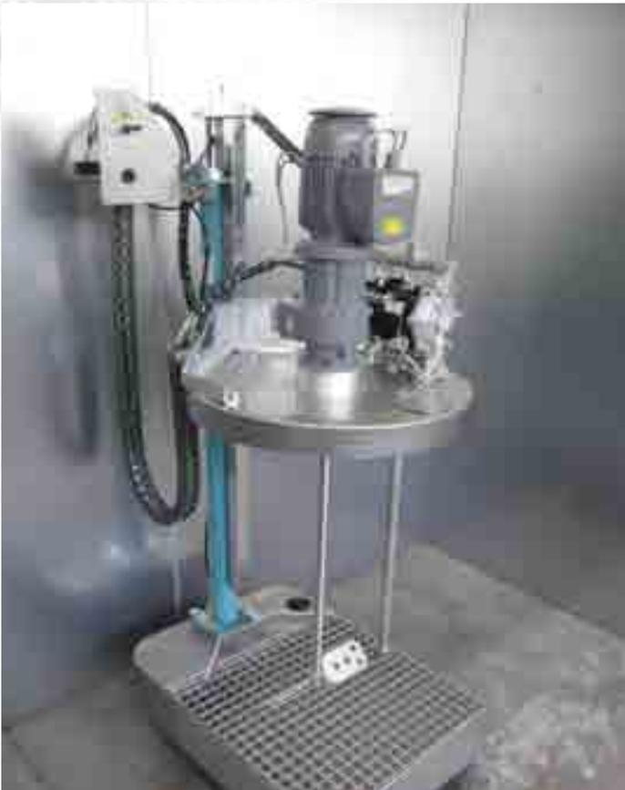
FU-ERW with brace, pump extraction from drip pan
