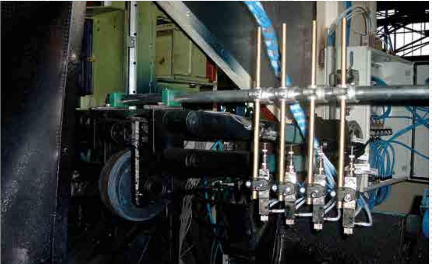
System with 4 paint colours for pipe marking
