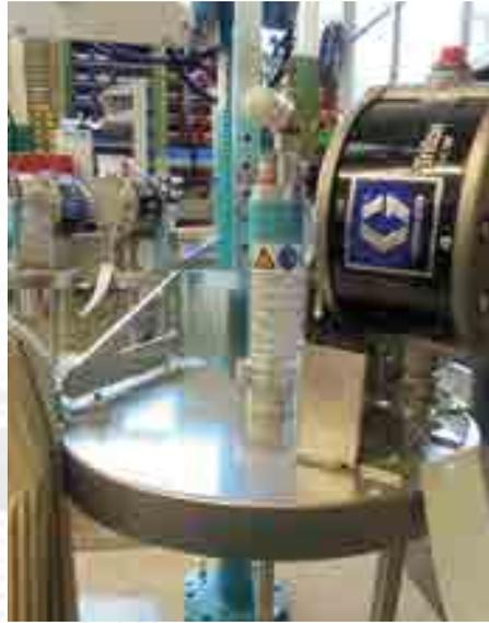
Agitator station 30 liters supply unit with diaphragm pump
