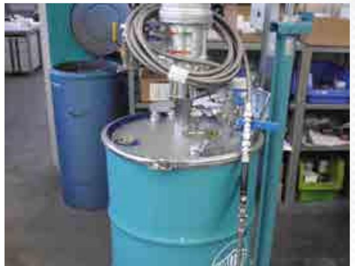
Material supply with clamp-on cover drum
