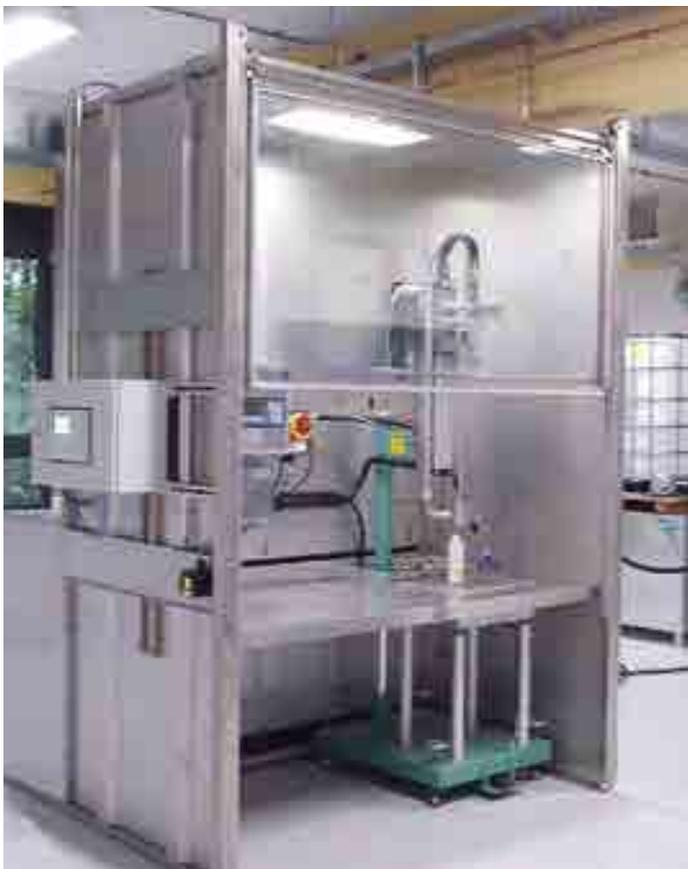
Filling of flammable liquids in bottles in exhaust cabin
