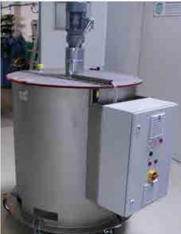
Mixing tank with electrical control
