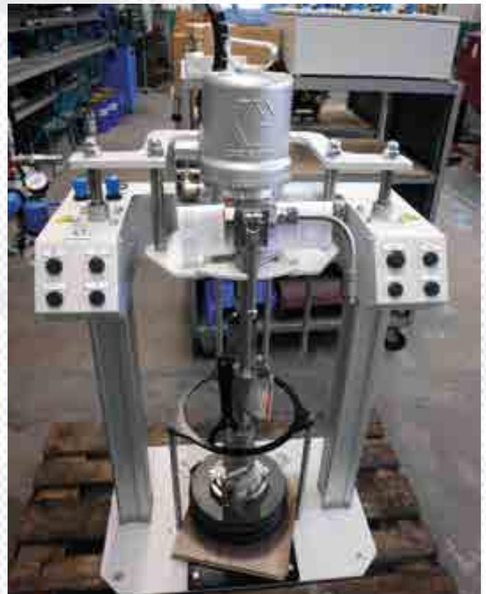
Pump station follower plate with two wiper rings **Part No. K 61 203 051 31**
