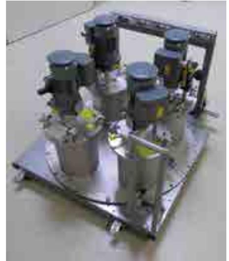
Split paint supply: This element is positioned under the conveyor line
