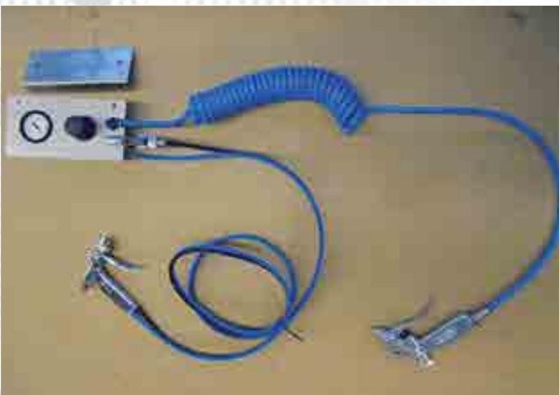
Release agent withdrawal station with blow-out gun Part No. 23 721 17
