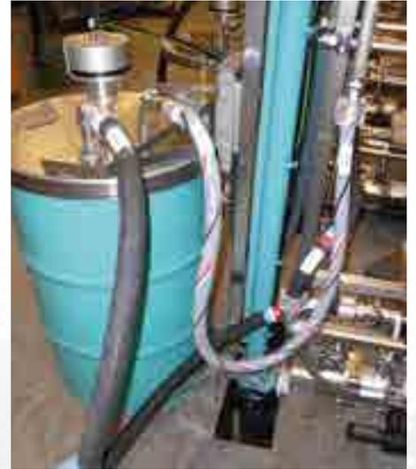
Material supply unit with agitator and horizontal plunger pump
