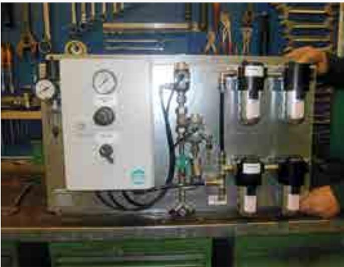
Mounting plate for desiccant bead filter, 2 flushing guns and detergent distributor
