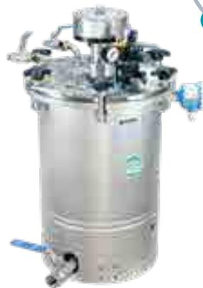
MDG 45 KLA with air-driven type 46-735 agitator along with tuning fork sensor to protect against overfilling. Fill at the bottom valve. The two upper valves for material recirculation - feed and return.
