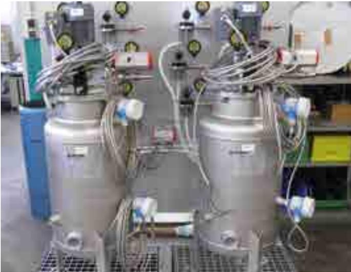
Material supply for 12 guns with pneumatically controlled material pressure regulators and digital pressure gauge
