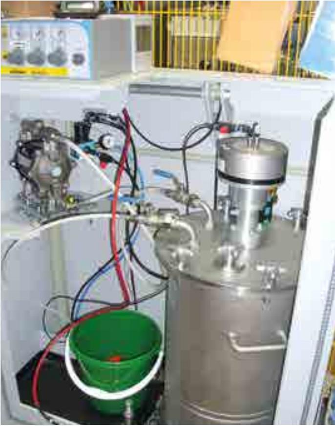
Aquacoat insulating cabinet with a pressure tank
