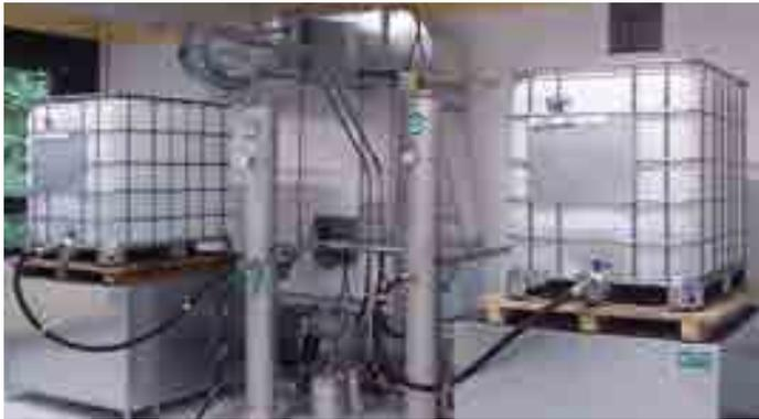
Material supply from containers / pump standpipe Part No. V 63 205 000 13
