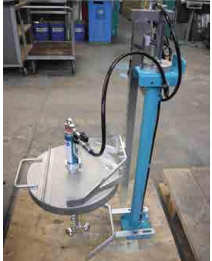
Agitated station with hinged cover and geared agitator Calix stirring element
