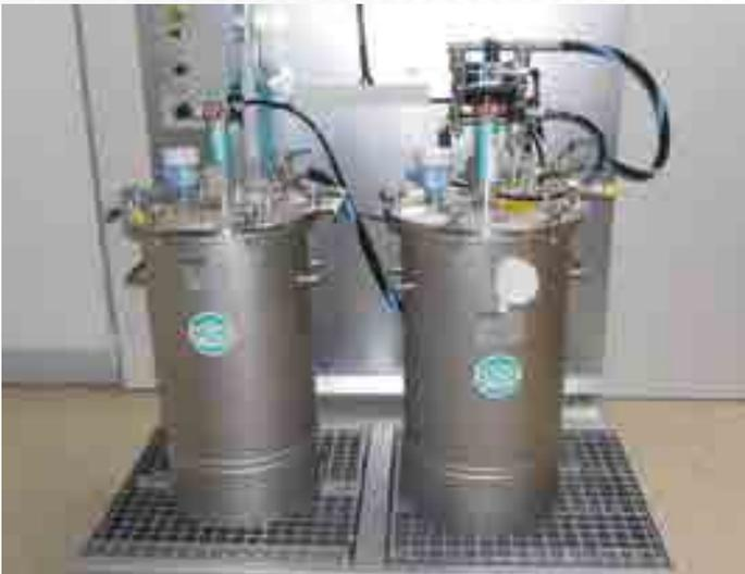
Material supply unit for moisture-sensitive material
