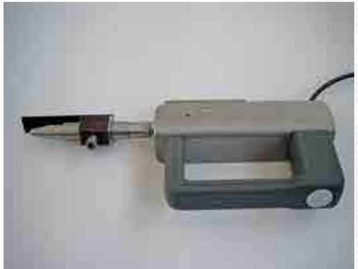
Extrusion gun WA 95 with manual trigger
