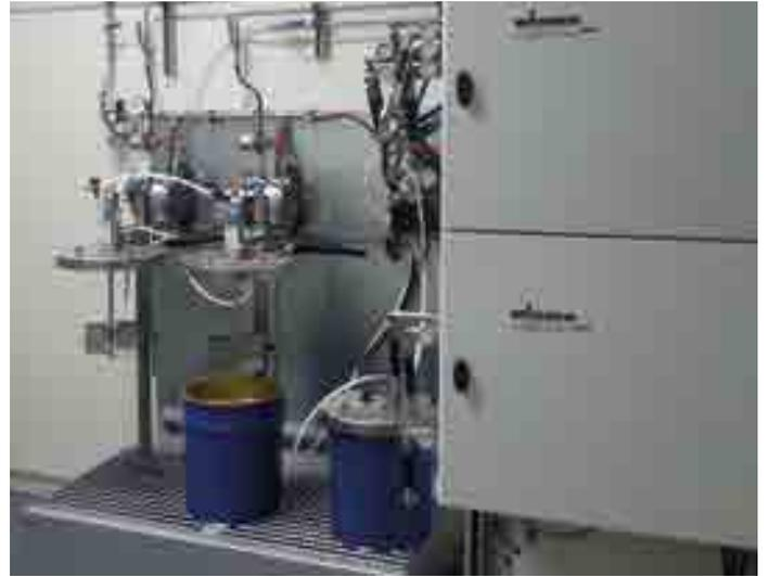
2K system material supply from pressure tanks
