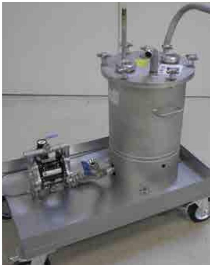
Trolley with pressure tank and circulation pump
