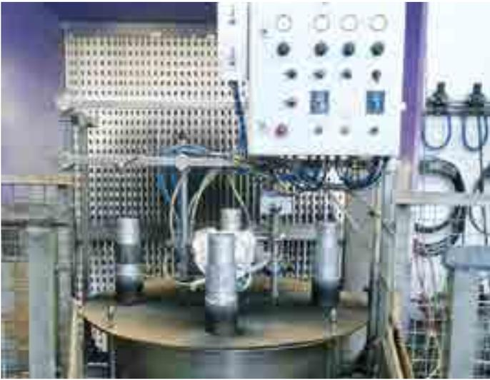
Spray table, revolving turntable with 4 workpiece holders
