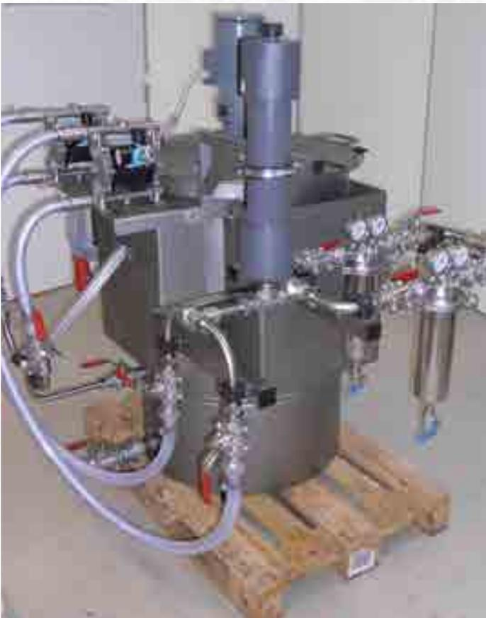
Mixing tank with pump pulsation damper and material filter system
