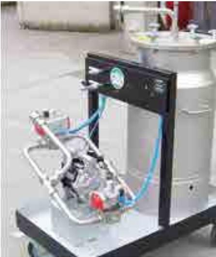
Trolley with pressure tank and diaphragm pump
