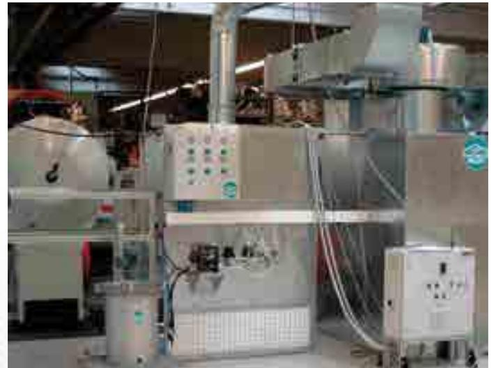
Material supply with mixing tank behind spray booth
