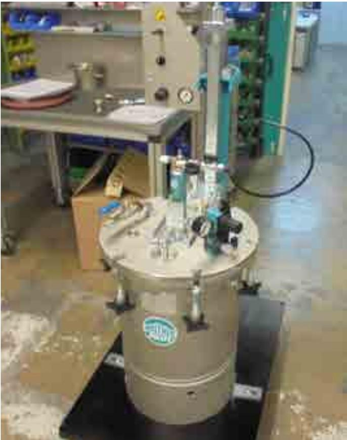
Pressure tank with pneumatic agitator
