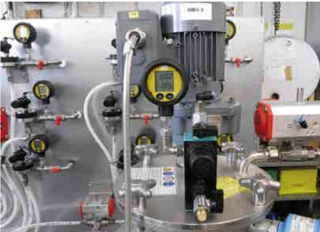
Pressure tank with electric pressure indicator
