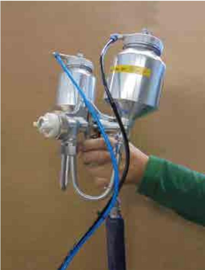
2-component hand gun for processing small quantities in the lab area
