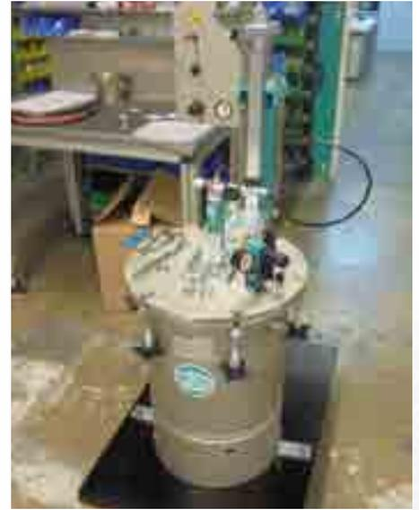
Pressure tank with pneumatic agitator
