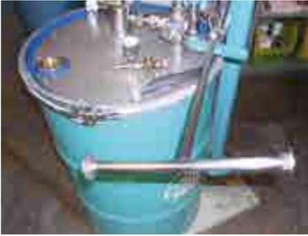
Drum with protective atmosphere applied to it
