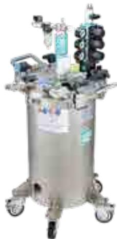
MDG 22 KLA with air-driven type 46-810 agitator, air inlet fittings with two additional regulators, as well as a splitter with two ball valves to connect two spray guns. The tank is equipped with castors and hand grips for portable use.
