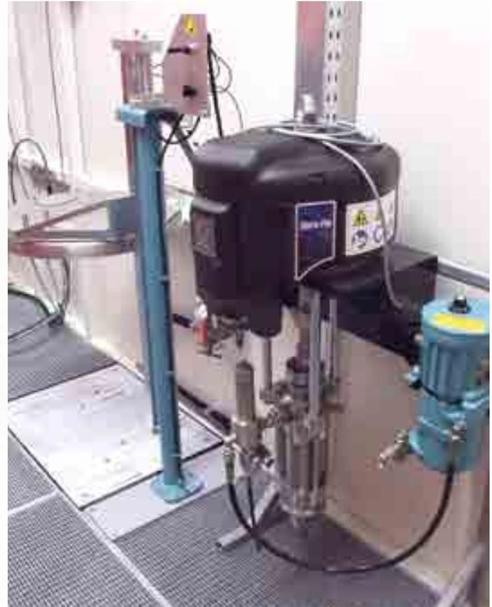
Pump station with electronic scales
