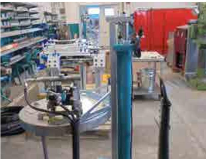
Drum cover lift with diaphragm pump for paint cabin ready for connection
