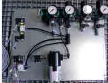
Simple air supply with desiccant bead filter on mounting plate
