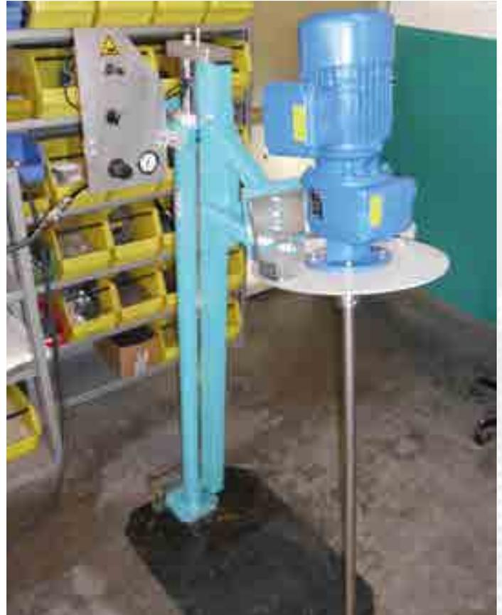
Agitator station with slanted shaft
