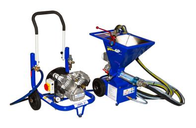
Spraying set composed of an EUROPRO 30+ compressor and an EUROPRO 4P, the most compact spraying machine on the market, with its 20 litres tank. Ideal for small jobs and touch-ups.
