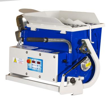
CP Joint 20, Machine compatible with CP 30, 35, 40, 45 & 55 Mixing type sequential Motor 1 1 kW 28 to 80 RPM Forward / reverse rotation speed 230 V - 10 A - 50 & 60 Hz Power supply Tank capacity 70 L Water meter integrated Mixing paddle double helical paddle Loading height 135 cm Dimensions (L x w x h) 88 x 52 x 57 cm Weight 75 kg
